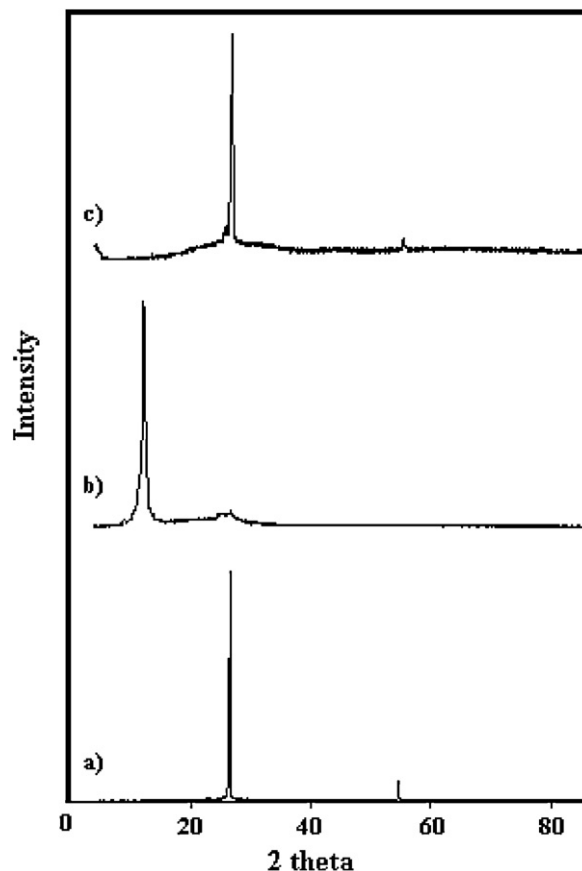
Fig. 3. X-ray diffraction patterns of (a) graphite (b) graphite oxide and (c) graphene.
